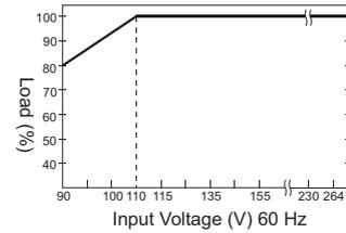
Figure 5 Relation between output power and input voltage
