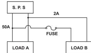
Figure 12: Output wiring
