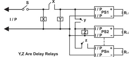
Figure 13: Delay circuit
