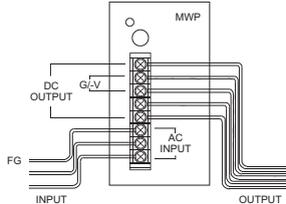
Figure 2 Wiring and connection
