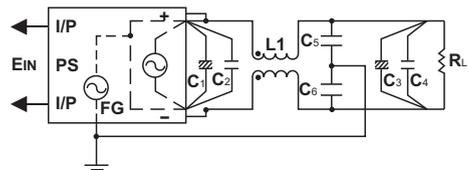
Figure 15: Ripple noise suppression
